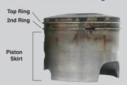
The piston rings earned a perfect merit rating, demonstrating no-stick performance. The piston skirts contained no scuffing, proving HP Marine's superior lubricity and friction-reduction capabilities.
