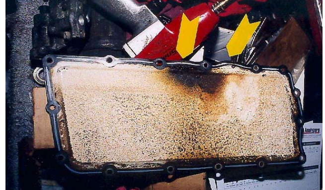
Figure 1. severe case of leaking plenum gasket
