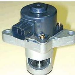
In either case, a malfunctioning EGR valve leads to drivability problems and loss of NOx control. Increased NOx results in rapid degradation of the engine's motor oil, including increased oil nitration, decreased ability to neutralize acids (TBN) and maintain internal cleanliness, oil thickening and/or sludge formation.
