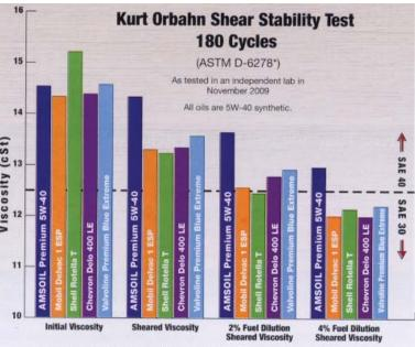
\*ASTM D-6278 specifies 90 cycles. AMSOIL requested a double-length test.
