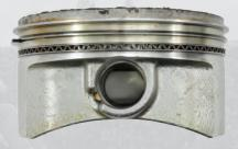
The piston and rings are virtually free of deposits and wear after 500 hours of severe-service testing in the Kawasaki\* FX 730 V engine.
