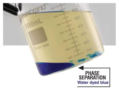
When ethanol/water mixtures fall to the bottom of fuel containers, it leads to lean-burn situations. Quickshot helps keep water molecules dispersed to prevent phase separation.
