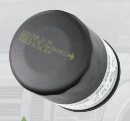
AMSOIL Oil Filters feature a reference arrow to aid in proper installation. Once the filter is finger tight, it is easy to gauge the additional .75 to 1.25 turns required to ensure a good fit. Over-tightening can lead to leakage.
