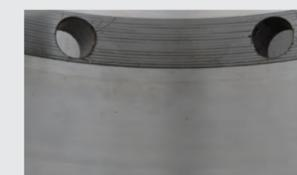
Following 512,000 miles, the transmission's output shaft bearing demonstrated no pitting or scoring despite frequent high-load operation. It earned a high wear rating of 8 out of 10, indicating only trace-light wear.
