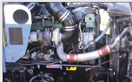
The Detroit Diesel Reliablite engine is still running strong after more than 1.1 million miles. The AMSOIL DUAL-GARD Oil Filtration System (lower left) allows for 100,000-mile oil change intervals.
