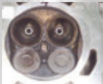
Combustion chamber before P.i.® treatment
