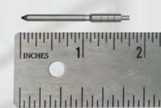
High-Pressure Common-Rail (HPCR) Fuel Injector Pintal
