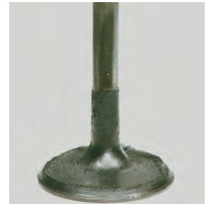
Picture E - Intake valve after P.i. treatment
