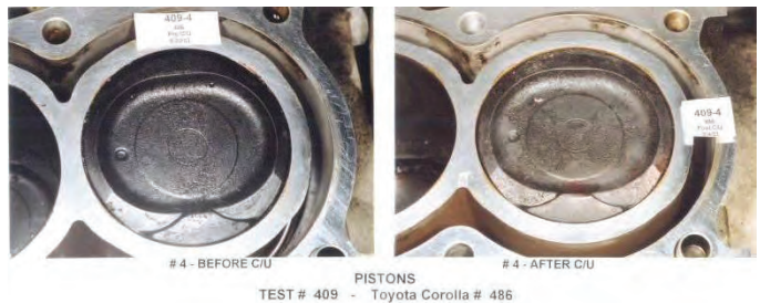
Picture G - Piston before P.i. treatment
