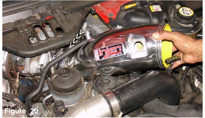
Figure 19 The cast intake is lowered and aligned with the 4" hose over the turbo inlet.
