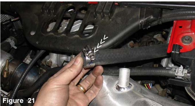
Important- Check for kinks in the ventilation hose. Any kinks in the line may cause cooling problems to the turbo if not checked prior to starting the engine. Figure 22 The clamp is now fastened over the 19mm hose as shown above. Once you have tightened the clamp, check to make sure there are no kinks in the line.
