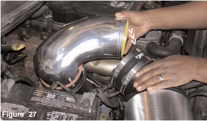
Figure 27 Once the intake has been align, continue to insert the intake into the plenum hose.
