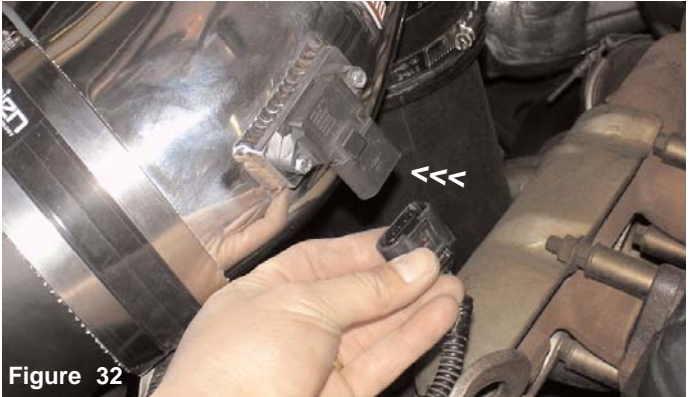
Figure 32 Press the electrical sensor clip over the MAFS until you hear them snap together.
