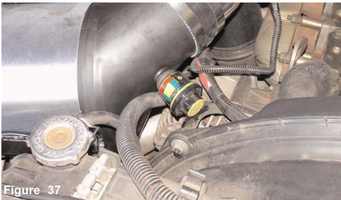
Figure 35 The air restrictor gauge is now installed in the plenum.
