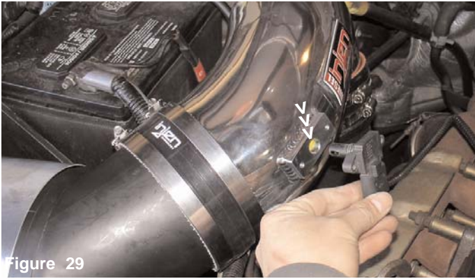
Figure 29 Insert the mass air flow sensor into the machined adapter. Prior to positioning the MAFS, rub a small amount of light oil on the O-ring to prevent the O-ring from kinking or ripping.
