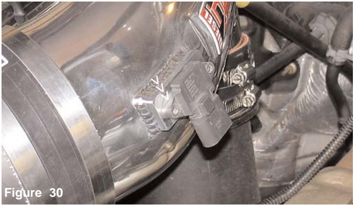
Figure 30 The MAFS is carefully pressed into the sensor adapter.
