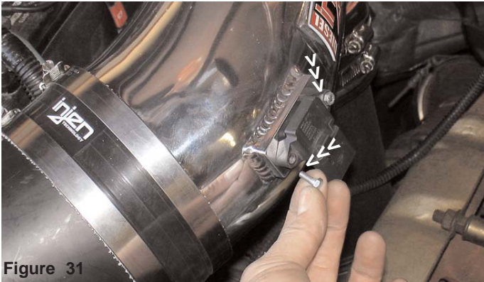
Figure 31 Use the m4 x 16mm button head screws to fasten the mass air flow sensor to the sensor adapter.
