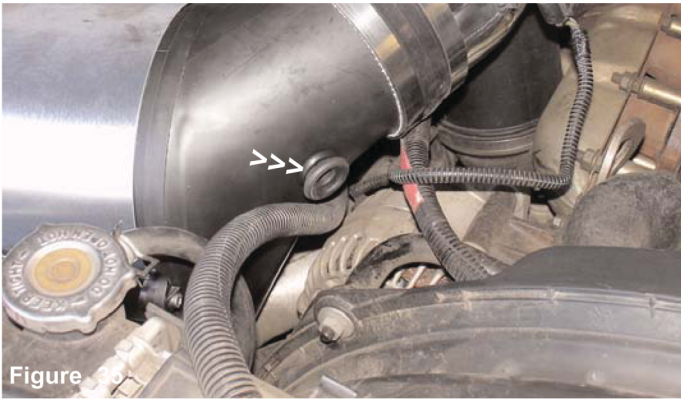
Figure 36 Press the air restrictor gauge into the Injen/AMSOIL grommet as shown above.
