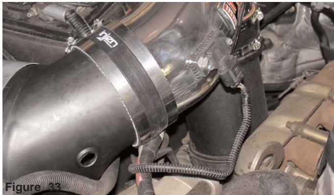
Figure 33 The electrical sensor clip is now firmly secured to the mass air flow sensor.
