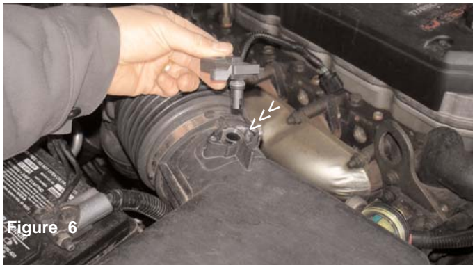
Figure 4 Depress the tab on the electrical harness clip and disengage it from the mass air flow sensor as shown above.
