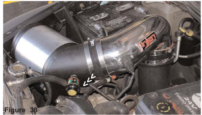
Figure 36 Press the air restrictor gauge into the Injen/AMSOIL grommet as shown above.
