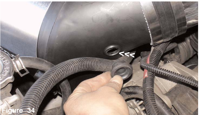
Figure 34 Press the new air restrictor gauge into the pre-drilled 3/4" hole on the plenum. Rotate the grommet so that the grommet is free from any lines.
