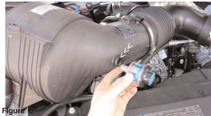
Figure 9 Pull the air restrictor gauge from the stock grommet as shown above.
