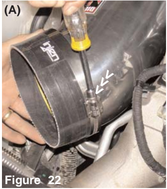
Figure 20 Once you have aligned the cast intake to the step hose, continue to press the intake into the hose (A) The power-band on the intake side is semi-tightened to hold the intake in place (B).
