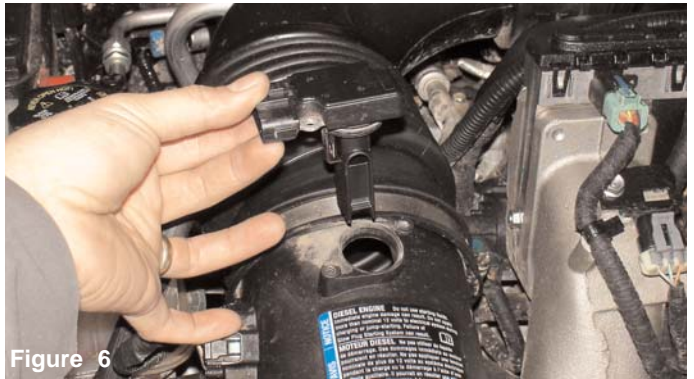
Figure 6 Once you have removed the bolts, continue to pull the mass air flow sensor out of the sensor housing.
