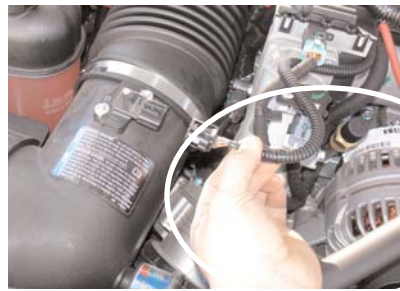
Depress the tab on the electrical harness clip and disengage it from the mass air flow sensor as shown above.
