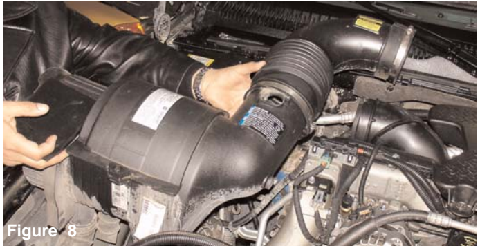
Figure 8 Once all clamps and hoses have been removed from the air box cleaner, continue to pull the entire air box out of the engine compartment. Pull up on the air box to disengage air box pegs from the grommets.
