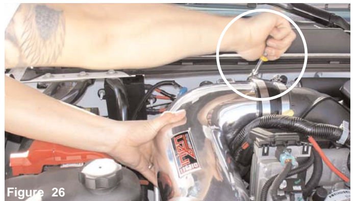
Figure 24 Once you have installed the straight hose over the end of the intake, continue to press the hose over the intake plenum.
