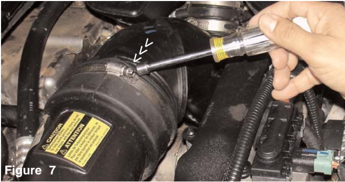
Figure 7 Loosen clamp on the turbo inlet tube connected to the air intake duct.
