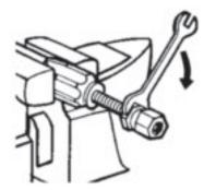
3. Screw nipple assembly into socket using wrench on nipple hex until nipple hex shoulders against socket.
