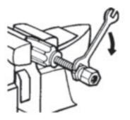
Screw nipple assembly into socket using wrench on nipple hex until nipple hex shoulders against socket.
