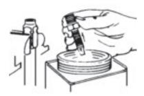
2. Oil inside of hose and nipple threads liberally with oil. Do not oil hose cover.
