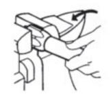
1. Place socket in vice and screw in hose counter-clockwise until hose bottoms. Back hose out ½ turn.
