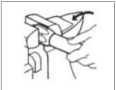
Place socket in vice and screw in hose counter-clockwise until hose bottoms. Back hose out 1/2 turn.
