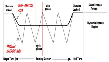
This line represents the effect a friction modifier has on maintaining the dynamic friction characteristics while in the slip phase and not allowing the resistance to build back up to the stick phase until the unit stops turning. At the same time, it helps to insure maximum power transfer to the wheels. The friction modifier additive can be thought of as a friction "controller," insuring maximum clutch pack engagement while allowing the conversion from lock to slip to occur gradually.
