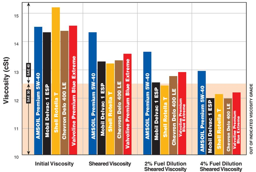
\*Oil diluted with fuel is especially prone to the effects of shearing. When combined with shearing conditions, as little as 4 percent fuel dilution is generally enough to reduce an oil's viscosity to less than the specified viscosity grade. Considering the tough environment that diesels present to lubricating oils, AMSOIL doubled the standard Kurt Orbahn 90-cycle test and had the oils tested for 180 cycles. Samples were then contaminated with 2 and 4 percent ultra-low-sulfur diesel fuel (ULSD).
