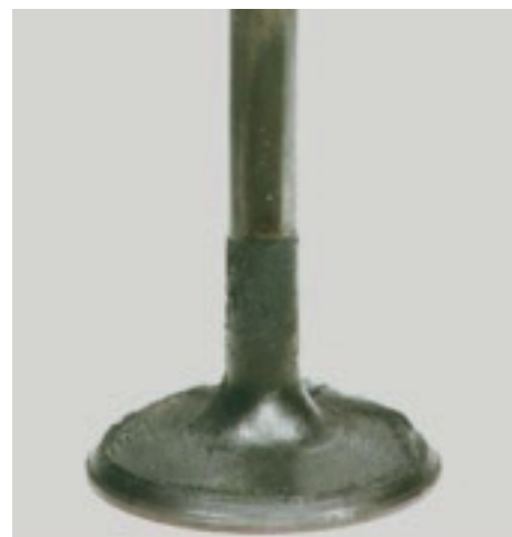
Picture E - Intake valve after P.i. treatment
