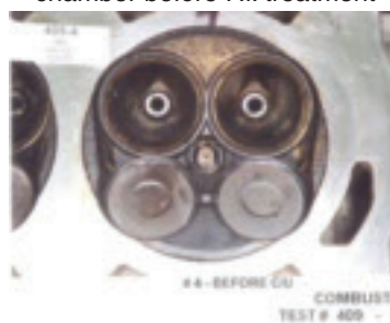
Picture F - Combustion chamber before P.i. treatment
