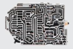
The transmission's valve body remaine clean and virtually sludge-free following more than 180 000 miles of severeservice driving Signature Series Synthetic ATF's anti-heat formulation provides dependable protection in severe
