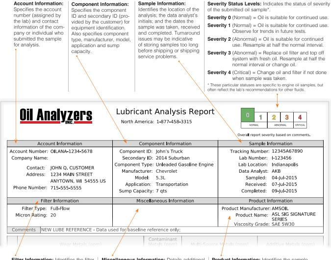
Filter Information: Identifies the filter used and its micron rating.
