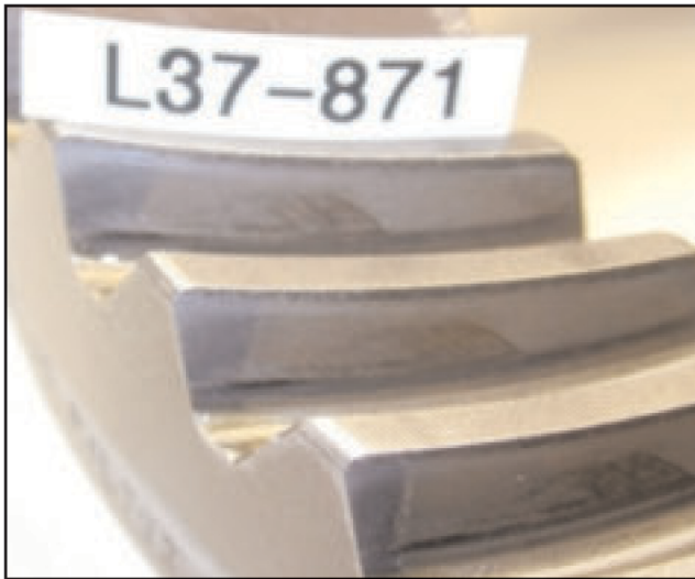
Ring gear exhibits very low wear.
