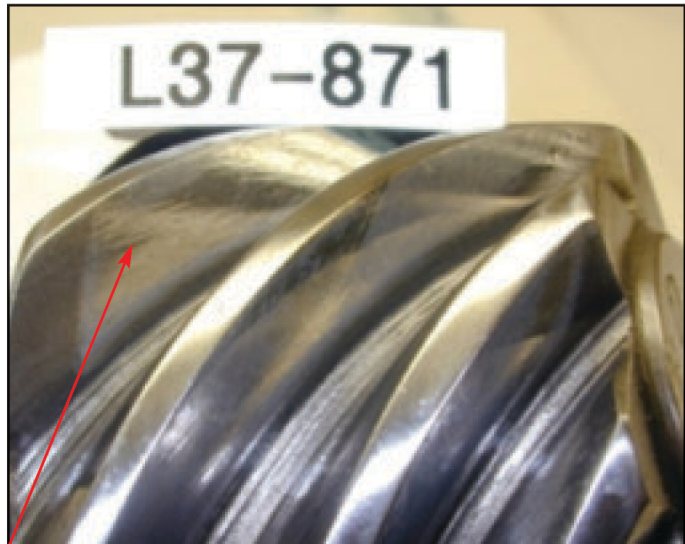
Pinion gear - original machine marks still present.
