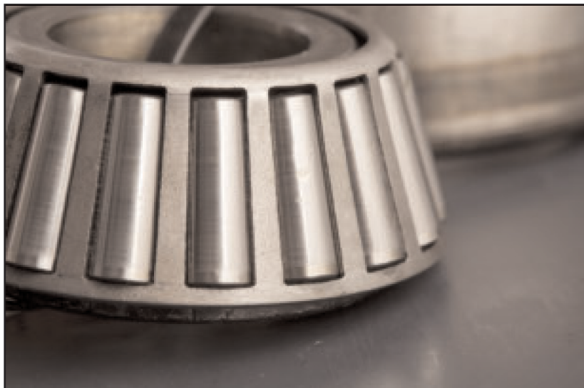
Pinion tapered roller bearing in like-new condition.
