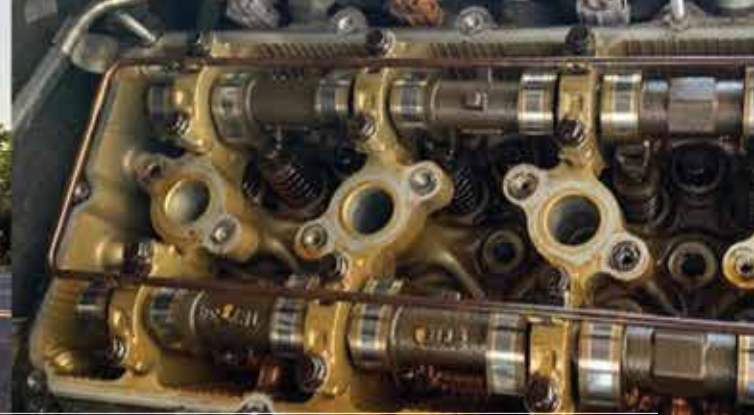
The valvetrain area is clean and void of excessive deposits or varnish, demonstrating the oil's excellent protection.
