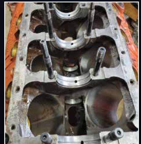
After 13 years of drag racing, the bearings in Jordan's Chrysler 408 showed virtually no signs of wear.
