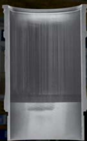
Severely Scuffed Liner
