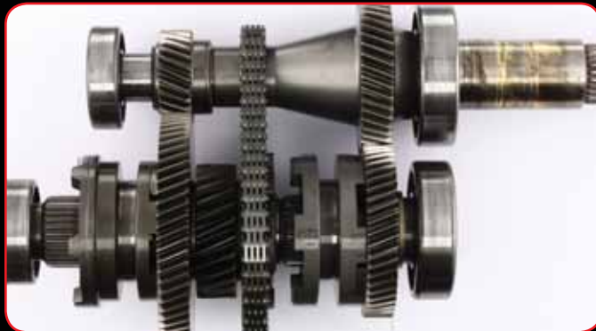
The transmission gears are in excellent condition and appear like-new despite the extreme heat.
