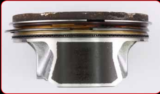
The piston skirt contained no scuffing and appears like-new, while the piston crown demonstrated no abnormal deposits following 100 severe-service hours.
