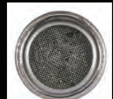
The oil pick-up tube screen is virtually free of sludge.
