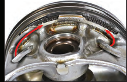
Example of piston damage due to an LSPI event observed during the testing of a competitor's motor oil. The red arrows indicate sections of the ring land that have broken away from the piston.
